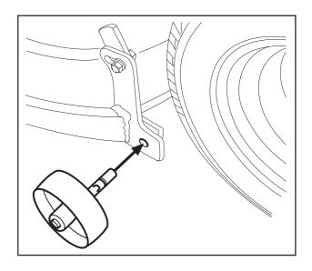
5. Disengage the spring from the drive belt tensioning wheel.
